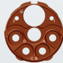
7-polig Stift 7-pin male 5 x Ø 2 mm (4+PE) + 2 x Ø 1 mm
