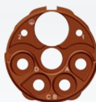
7-polig Stift E Code 8 7-pin male contact E Code 8 (5 x Ø 2 mm (4 + PE) + 2 x Ø 1 mm)
