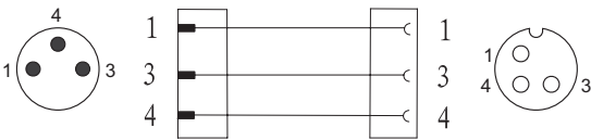
3 Poles Contact assignment of M8 to M12 T1 connector
